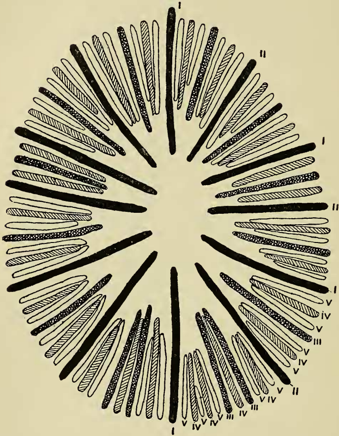
Diagrammatic plan of the septa of Paracyathus cavatus . The primary and secondary septa are black, the tertiaries are cross-hatched, the quaternaries are crossed with diagonal lines, the quinquaries are left blank; i, ii, iii, iv, v, septa of the first, second, third, fourth, and fifth cycles.
